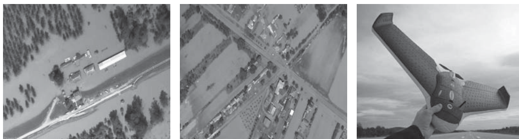
Figure 12 Detection of floods with a help from UAVs „Sensefly eBee“ – Bosut and Jamena (Source: Vojvodina waters, 2014)
