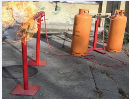
Figure 6 – Testing extinguishing at gas installations
