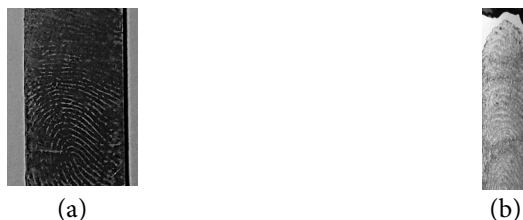
(a) (b) Figure 11. Electrodeposited nickel films on stainless steel substrates with 50 mA/cm 2 current density for: (a) 30 s, (b) 1 min.
