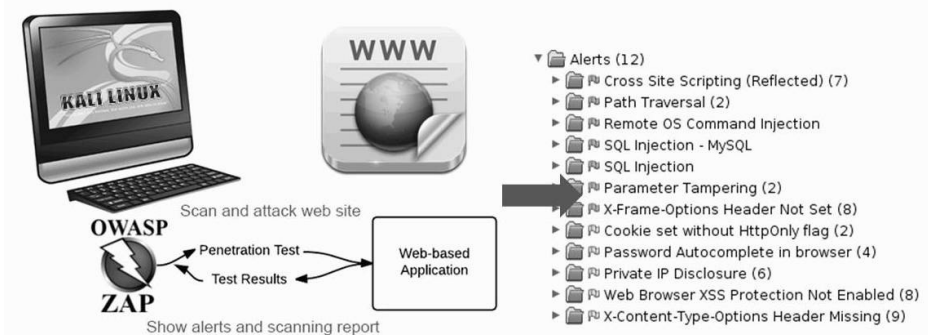
Figure 1. Framework for path traversal attack technique.
