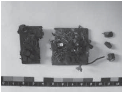
Figure 13: Car alarm fragments
