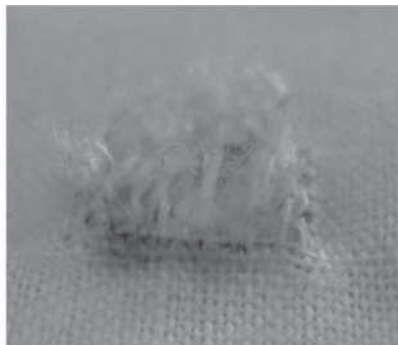
Fig. 11: Observed from the side of 79-micro submachine gun blunt bullet exit hole
