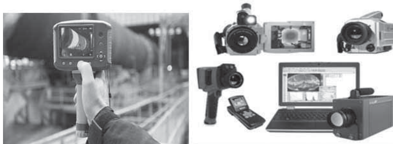
Figure 2. Thermal imaging equipment
