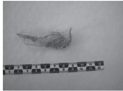
Figure 14: Enamelled wire fragments
