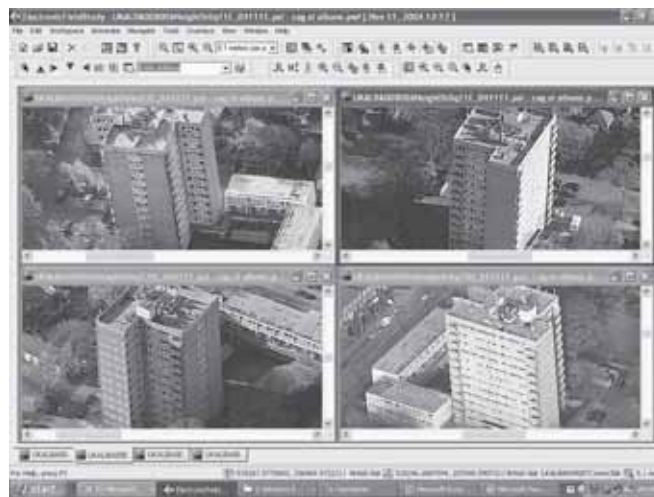
Figure 10. Independent software tool EFS (Electronic Field Study) for viewing and measurement (Source: Geo Info Strategies)
