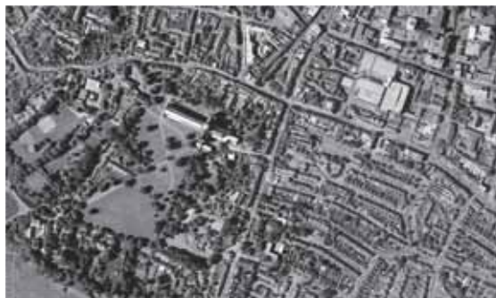
Figure 7. Classic orthophoto provides the view of the terrain from above (Source: Geo Info Strategies)
