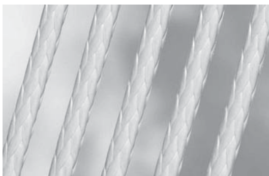
Figure 10 Microscopic appearance of Dyneema ® fibers
