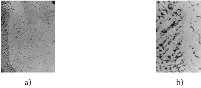
Figure 3.2: The microstructure of the longitudinal section of cord 3 with magnification of a) 56 b) 224
