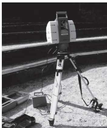
Figure 1. LIDAR installed on a stand or a SUV (Source: Wikipedia)
