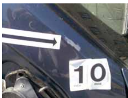
Fig. 6: The magnified paint damage
