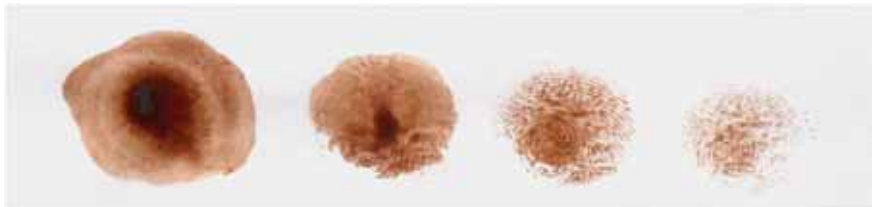
I II III IV Fig.2 Patent prints deposited four times successively with an amount of 20 \mu l human blood.
