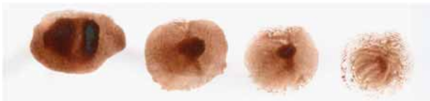
I II III IV Fig.4 Patent prints deposited four times successively with an amount of 40 \mu l human blood.
