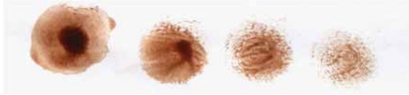
I II III IV Fig.1 Patent prints deposited four times successively with an amount of 15 \mu l human blood.
