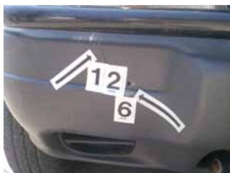
Fig. 7: The damage of bumper – slashes (12)
