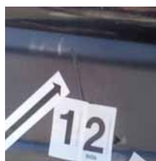
Fig. 8: Evidence no. 12 – part of blue fibre in slashes on the bumper
