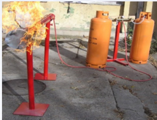
Figure 6 – Testing extinguishing at gas installations
