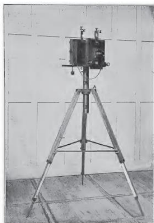
FIG. 1. — Apparatus of the Criminal Department (Bertillon model) for metric photography (judicial, forensic-medical, anthropological, etc.)
